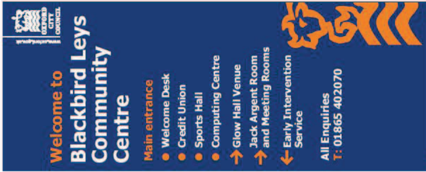
1.0 Front facing road Internally mounted post monolith 2500mm x 1000mm; approx 100mm returns (5000mm x 900mm is an off-shelf item) 500mm of 80mm posts in ground. Powder Coated RAL 5002 vinyl graphics artwork supplied
